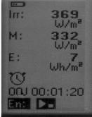
Irradiation, average, accumulated energy, Min./Max instantaneous irradiation
