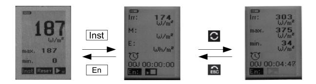
From start screen, the operator have access to energy measurement over a period controlled by timer and clock, he proceeds as follows:
