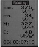
Irradiation, average, accumulated energy, Min./Max instantaneous irradiation
