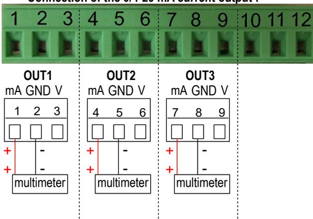
Connection of the 0/4-20 mA voltage output :
