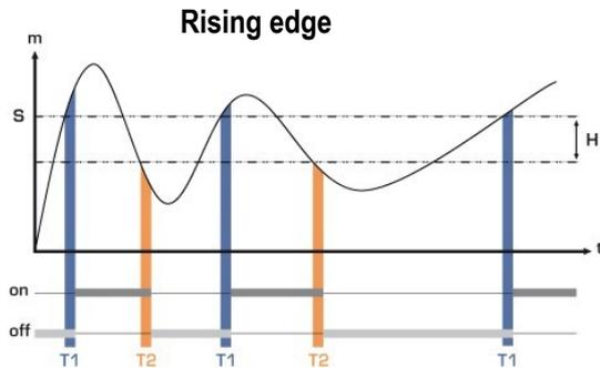
Measurement ( $m$ ) > Threshold ( $S$ ) during the time-delay  $T1$  → Alarm activation
