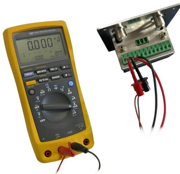
Connection of the 0/4-20 mA current output :
