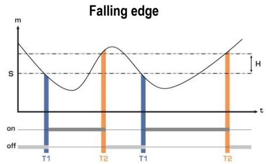
Measurement ( $m$ ) < Threshold ( $S$ ) during time-delay  $T1$  → Alarm activation.
