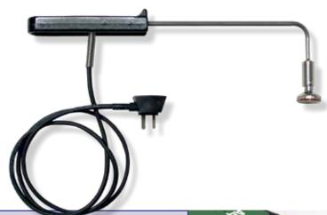
WRAP & STOW PROBES CAN BE REPLACED AT YOUR LOCATION AND MAINTAIN THE TOTAL SYSTEM ACCURACY WITHOUT CALIBRATION.
