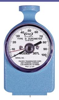
ASTM Type D Durometers are for determining indentation hardness of Pipeline Coating, Hard Rubber, Acrylic, Delrin, Kevlar, PVC, Nylon, Lexan and Epoxies.
