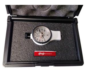
PTC Metrology<sup>™</sup> is accredited by A2LA for durometer calibration to ISO/IEC 17025. NIST traceable certification is available for all durometer types covered by current ASTM D2240, ASTM F1957, ISO 868, ISO 7619 and DIN 5305 standards.
