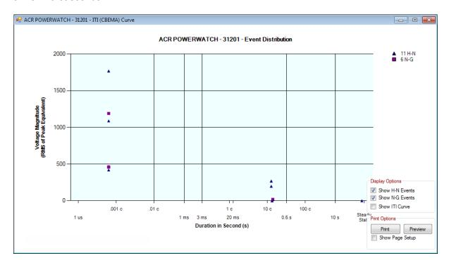
The ITI Curve has a maximum value of 500% of the nominal voltage. Events exceeding this value are not shown on the ITI curve. A message will appear at the top of the graph if this situation occurs.
