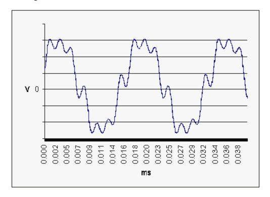
PowerWatch synchronizes itself to the consecutive positive and negative zero crossings of the AC line (every 8.33 milliseconds at 60Hz). Should the voltage waveform be so highly distorted that unexpected zero crossings are detected, PowerWatch will report a loss of synchronization relative to the measured voltage waveform.
