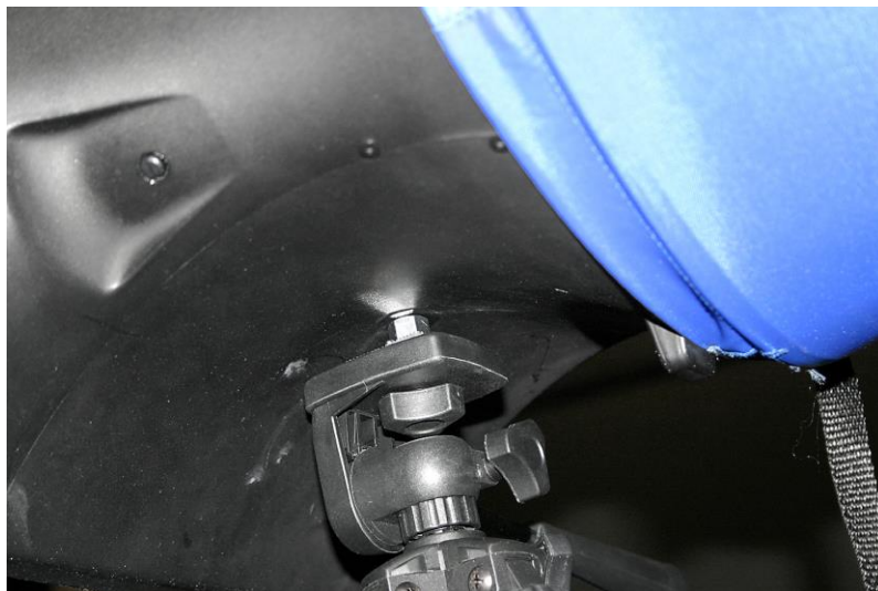
Figure 27: Mount Hood Base to Telescopic Stand
