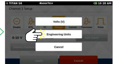
Select Engineering Units
