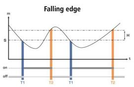
Measurement (m) < Threshold (S) during time-delay T1  $\rightarrow$  Alarm activation.
