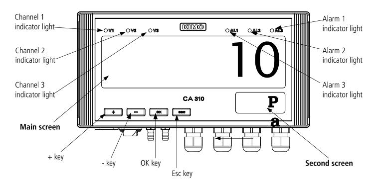
Main screen displays the measured values and the folders numbers. Second screen displays the measurement units and the sub-folders numbers.
