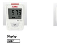
Set the protected mode of the KISTOCK\* "ON" or "OFF" by clicking ON\_OFF If the protected mode is activated, the measured values will not be displayed on the data logger. To deactivate the protected mode, set it on "OFF" or press for 3 seconds the "Selection" key of the data logger.
