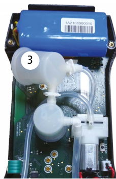
Sensor removed from white rubber cap
