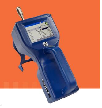
The TSI AeroTrak® 9306 Handheld Particle Counter offers the most features and flexibility for customers interested in versatile handheld particle contamination monitoring.
