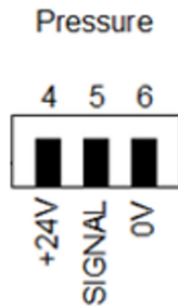
Figure 7 Pressure Sensor Connections
