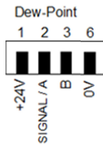
Figure 6 Dew-Point Sensor Connections
