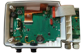
The wireless communication module is correctly inserted.
