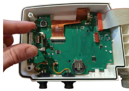
Hold the wireless communication module between your fingers as shown on the picture and slide it between the two holders.
