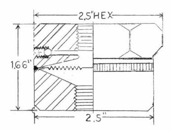
The 25AW seal is designed for use on up to 4 1/2" bourdon tube gauges, including most process gauges, with pressure ranges from vacuum to a maximum operating pressure of 1000 PSI at 100 degrees F.
