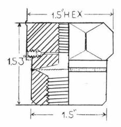
The 15AW mini-seal is designed for use on up to 3 1/2" bourdon tube gauges with a usual minimum range of 0-100 PSI.\* The maximum operating pressure is 2000 PSI at 100 degrees F.
