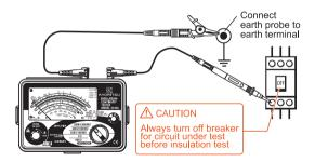
④ Check the circuit under test is not energized as follows.
