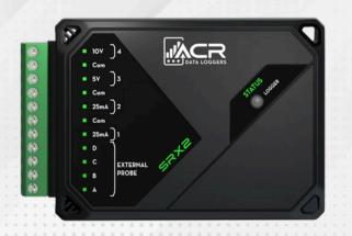
SRX2 is a self-powered, multi-channel data logger that can monitor and record temperature and relative humidity onboard and remotely, plus a variety of popular Process Signals at rate of 20 samples per second to 24 hours per sample. Includes TRX Basic software and Mini USB interface cable.
