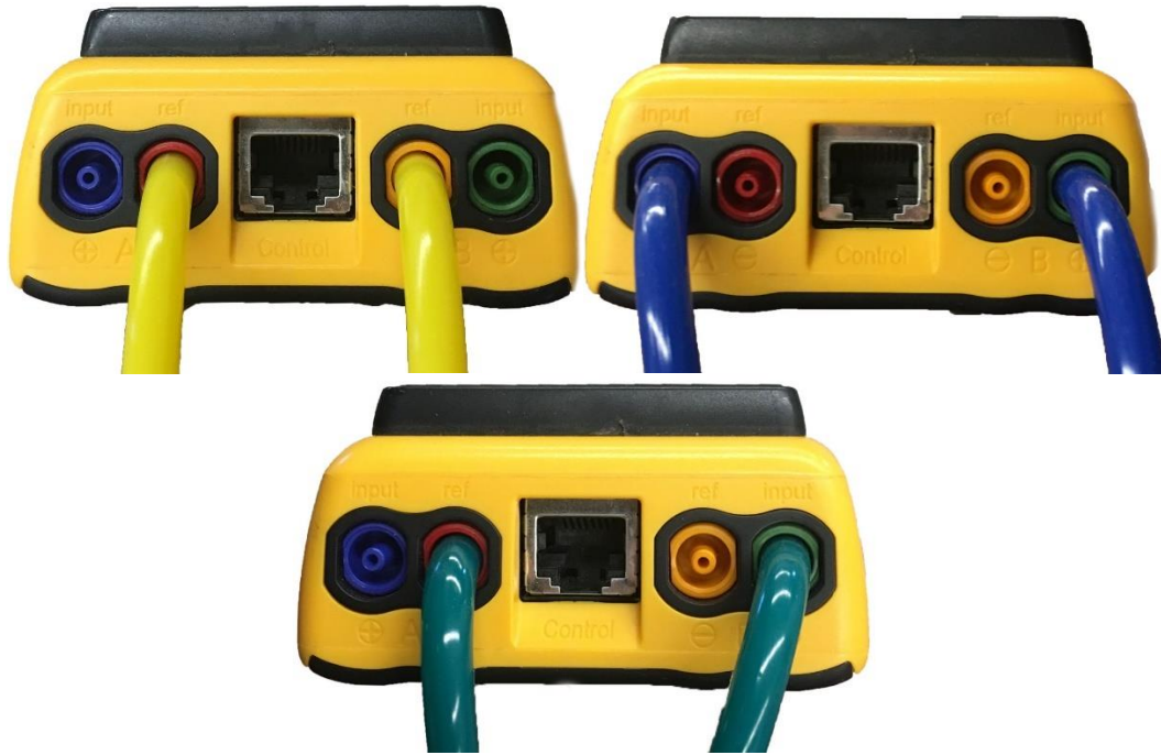
Yellow tube between Channel A & B. Blue tube check of positive ports. Green from negative to positive ports.
