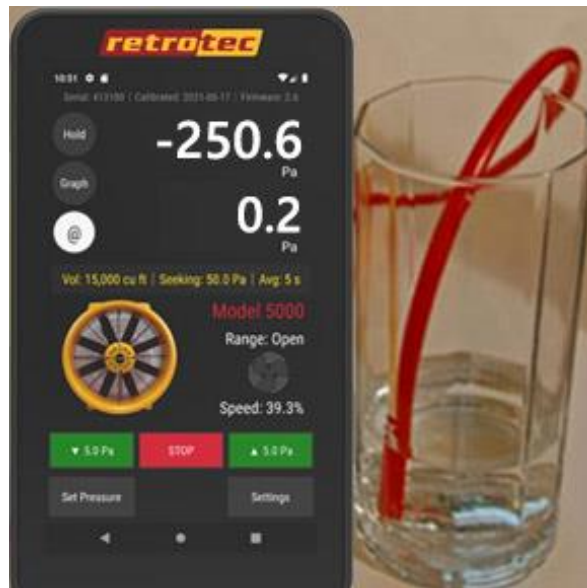
The gauge displaying a negative pressure (-250.6 Pa).
