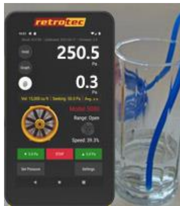
Gauge displaying 250.5 Pa (or 1 in WC).
