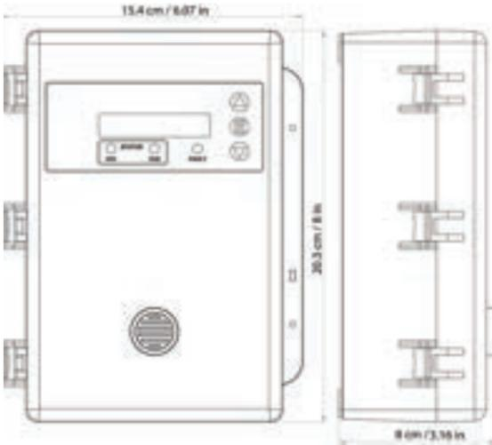
Note: Drawing above is shown without a splash guard. With the standard splash guard (Option -S), the thickness of the unit is 8.9 cm / 3.5 in and IP54 rated. With the splash guard for sticky gases, (Option -SN), the thickness of the unit is 12.6 cm / 5.02 in.
