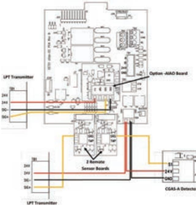
Three-conductor, 16 - 18 gauge wire / cable must be shielded when connecting to a remote analog transmitter. The LPT and CGAS-A series of remote analog transmitter enclosures have several conduit entry locations (general purpose enclosure).
