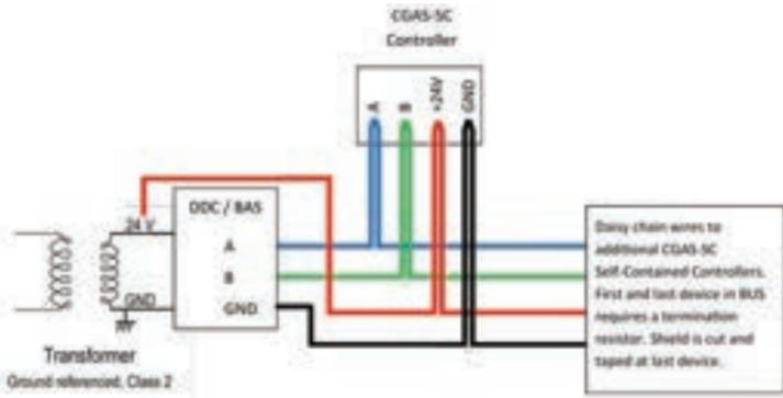
**Wiring Example: 4-Wire VDC**
