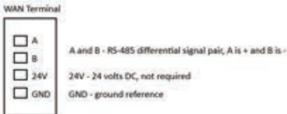
The wiring between the cGas-SC and a controller or BAS/DDC or multiple cGas-SC devices, should be 4-conductor shielded 16 awg stranded within conduit in a network wiring (daisy-chain) configuration. Suggested 4-conductor, 16 AWG, shielded stranded wire cable types are AlphaWire 79220, Belden 5202FE 008500 or equivalent.
