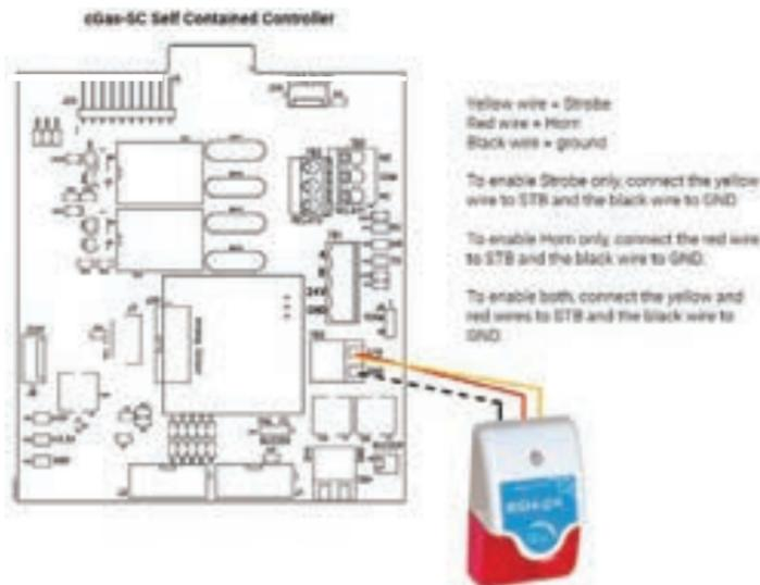
Alternatively, the remote horn/strobe can be connected to one of the cGas-SC relays, especially if multiple remote horn/strobes are needed. Note: This method requires a separate power source as the relays DO NOT supply power. See Section 4.10 Relay Connections for more information.
