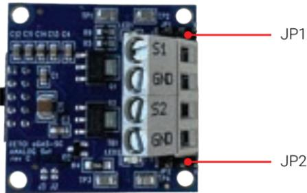
Find JP1 and JP2 on the 2AO board and move the jumpers as indicated by the black area for current and voltage.
