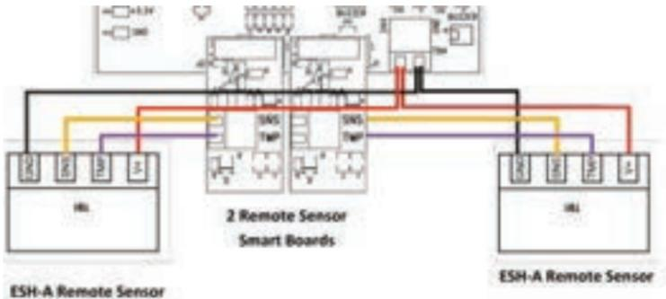
**NOTE:** The ESH-A Remote Sensor has a temperature sensor which should be wired to the TMP position.
