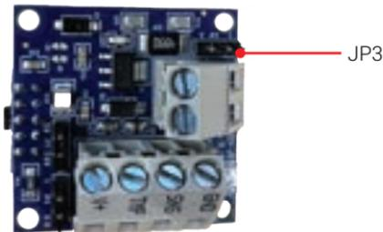
Find JP3 on the board and move the jumpers as indicated by the black area for current and voltage.
