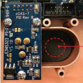
When installing a second smart sensor after initially ordering a single smart sensor model, you will need to remove the center circular cut out of the foam in the second sensor vent area before installing the smart board.
