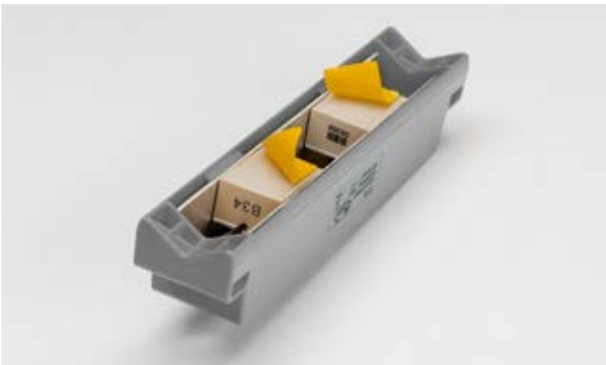
Figure 12 Applying the gel pads
