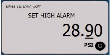
Once the alarm setpoint has been reached the high or low alarm icon will show on the display and background color will change to red to indicate an alarm status.
