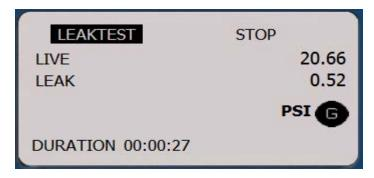
To stop the test at any time, press right arrow to highlight STOP. When the test is complete, the gauge will display the leak rate in units/minute. In addition, the results with start time and end time are displayed until the next test is started. Minimum test time is 10 seconds. To start a new test, use the left arrow key.
