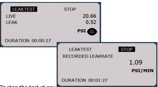
To stop the test at any time, press right arrow to highlight STOP. When the test is complete, the gauge will display the leak rate in units/minute. In addition, the results with start time and end time are displayed until the next test is started. Minimum test time is 10 seconds. To start a new test, use the left arrow key.
