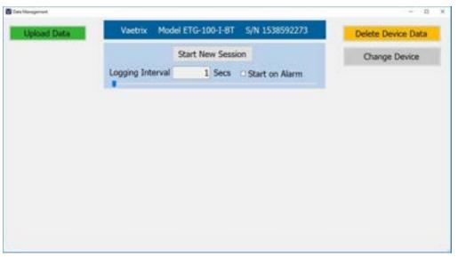
To start a new session simply use the slider bar or type in value to set the logging interval from one second to twenty-four hours and the press the Start New Session button. A session can be ended at any time by clicking Stop Session. If the High or Low Alarm values are enabled in the ETG, datalogging can be started automatically.
