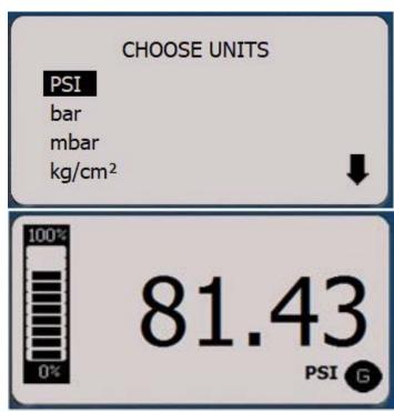
Press the UNITS key to accept the selection and the gauge will return to *Measure Mode*.
