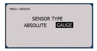
Absolute pressure is referenced to a perfect vacuum so it's equal the sum of Gauge pressure and Atmospheric pressure. Gauge pressure is always referenced to atmosphere. It is always crucial to perform a zero before attempting a calibration to eliminate any errors that may be caused by fluctuating pressure or changing conditions.
