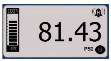
If you prefer not to use the bar graph, it can be turned OFF by using the RIGHT arrow key and pressing SELECT. *The bargraph will not be displayed with units measuring temperature.*
