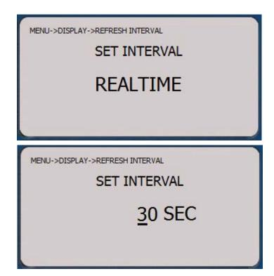
If a high update rate is not needed the interval can be extended to conserve battery life. To adjust the refresh intervals in seconds, use the Arrow Keys and press SELECT. The interval can be set to a maximum of thirty seconds.
