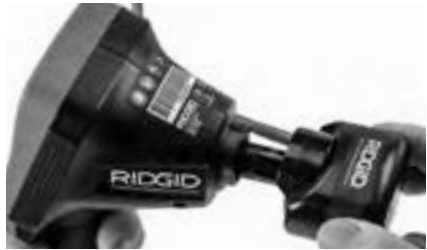
Figure 18 – Camera Connector Plug Installed
