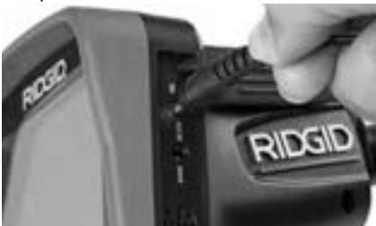
Figure 6 – Powering the Unit with AC Adapter
