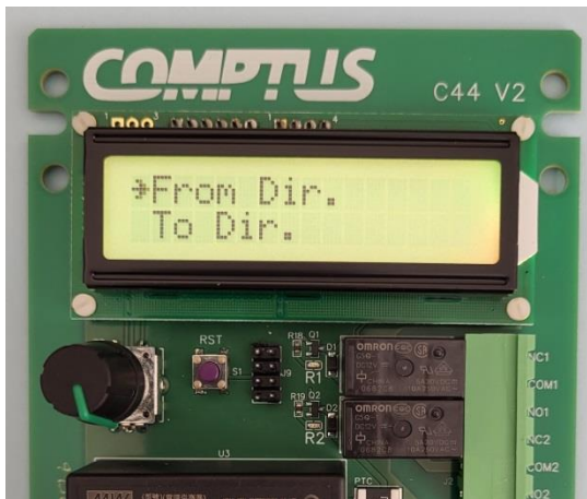
Use “From Dir.” to set start of arc to alarm
