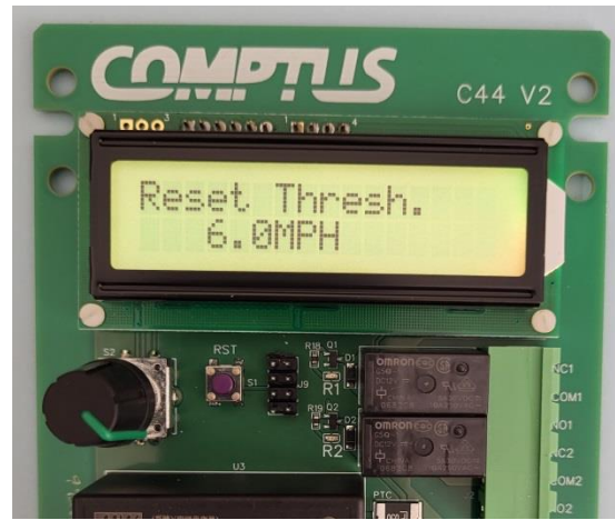
Select “Reset Thresh.” – alarm off speed
